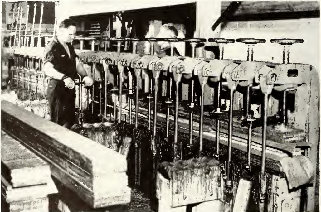
FIGURE 5-37.—A type of screw press used in gluing flat laminated stock.
